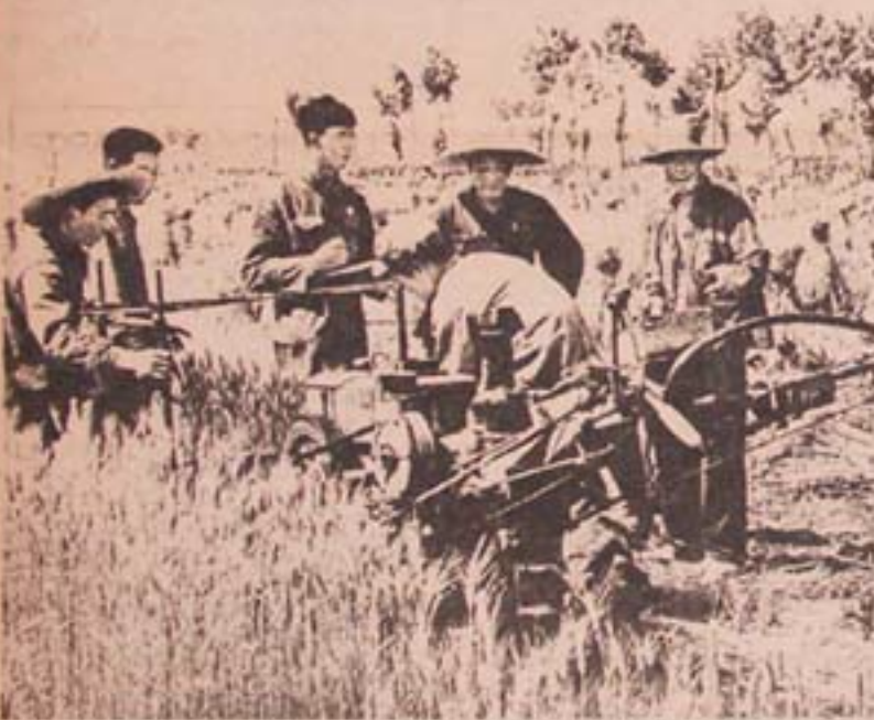
Personnel from a People's China county farm machinery research center and factory test a small harvester of wheat and rice.
